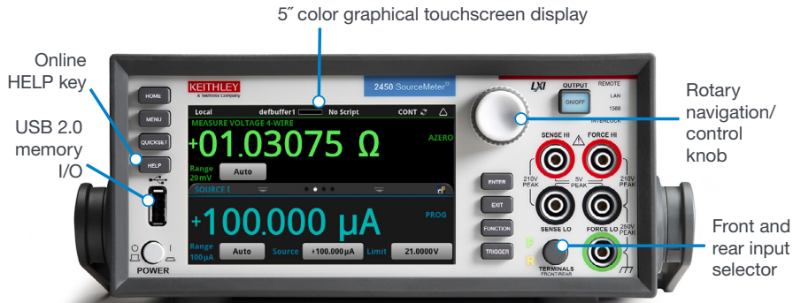
2450 front panel with high-resolution, capacitive touchscreen.
